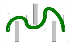
Figure 6. Approximation by Ferguson curve after changing the control point 4 (Pavlovkin)
