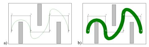
Figure 5. Approximation by Ferguson curve (Pavlovkin): a) for a pointwise vehicle; b) for a real vehicle
