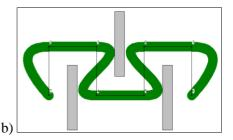
Figure 3. Interpolation by Bezier curve (Pavlovkin): a) for a pointwise vehicle; b) for a real vehicle
