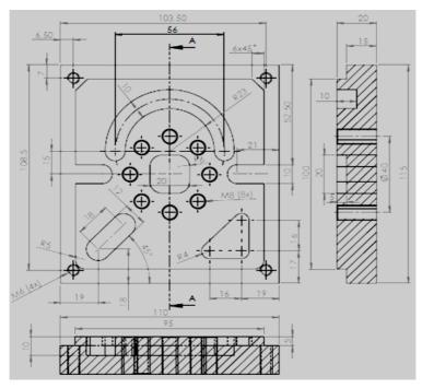
Figure 1. Designed component
