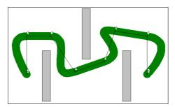
Figure 4. Interpolation by Bezier curve after changing the coordinates of the control points (Pavlovkin)
