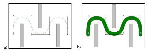
Figure 7. Approximation by Cubic B-Spline (Pavlovkin): a) for a pointwise vehicle; b) for a real vehicle
