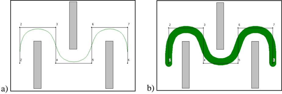
**Figure 7. Approximation by Cubic B-Spline (Pavlovkin):**
