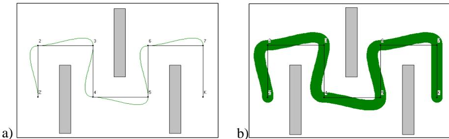
**Figure 2. Interpolation by Ferguson curve (Pavlovkin):**
